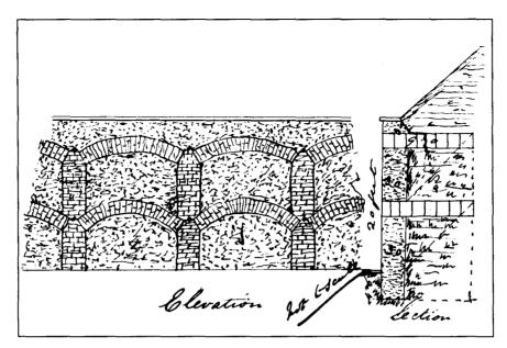
4 This sketch and those in Figures 5, 6 and 7 are from the series of reports written by engineer officers at Halifax describing their work with cement concrete. Here the use of concrete for the front wall of the scarp at Fort Charlotte is shown. In this wall the piers and arches, which were of masonry, were flush with the concrete, but it was suggested that it would have been an improvement to let them project. National Archives of Canada, RG8, C Series, Vol. 1587, p. 165.
