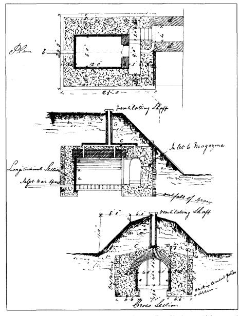
5 These sketches show the expense magazines at Fort Charlotte, which were of concrete lined with brickwork with an airspace between to help keep the magazines dry. *National Archives of Canada, RG8, C Series, Vol. 1587, p. 167.*
