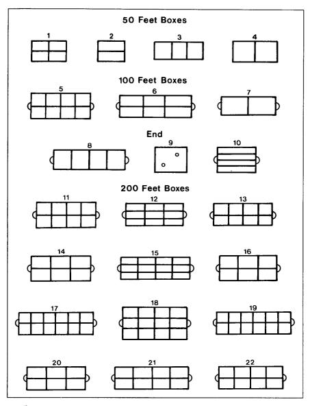
Boxes to contain 50, 100 and 200 feet of glass, showing where the divisions should be in the boxes for various sizes of panes and how the handles should be placed. *Redrawn by D. Sullivan from Cooper, Crown Glass Cutter and Glazier's Manual, 1835.*
