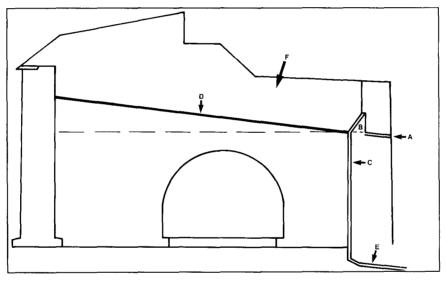
11 Holloway was using asphalt over the arches, but covered by earth, in conjunction with drains protected from the frost. (a) Old drain blocked up; (b) Masonry to lead water from the rear wall; (c) Drain through pier; (d) Line of gutter on dos d'âne; (e) Underground brick drain; (f) Earth covering. *Redrawn by D. Sullivan.*
