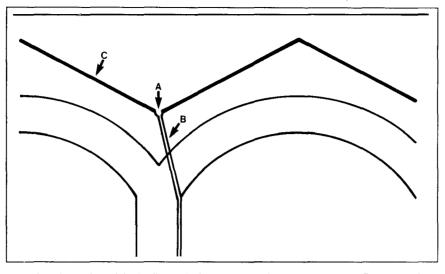
**12** Sketch enclosed in Holloway's letter of 23 June 1845 to the Board of Ordnance showing the work at Fort Henry, Kingston. (a) Internal drain; (b) Guttering of dos d'âne; (c) Asphalt covering of dos d'âne. *Redrawn by D. Sullivan*.
